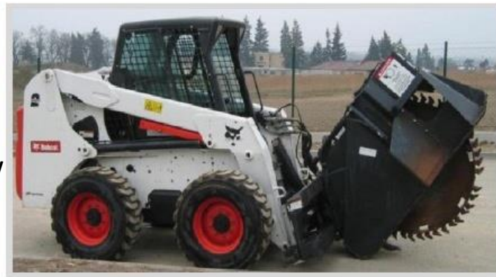
Bobcat: S750 Skid Loader with WS18/24 Wheel Saw
